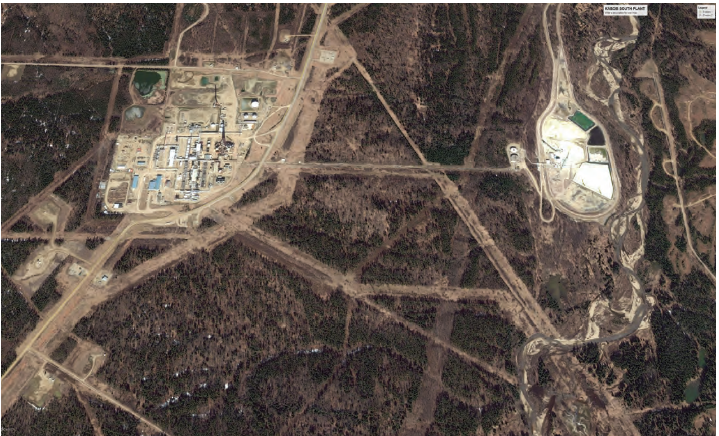
A satellite image of SemGroup’s Kabob South gas plant in Fox Creek, Alberta, which includes water-handling ponds, where waste brine is treated before reinjection into the subsurface. EMPIRE ROCK MINERALS
